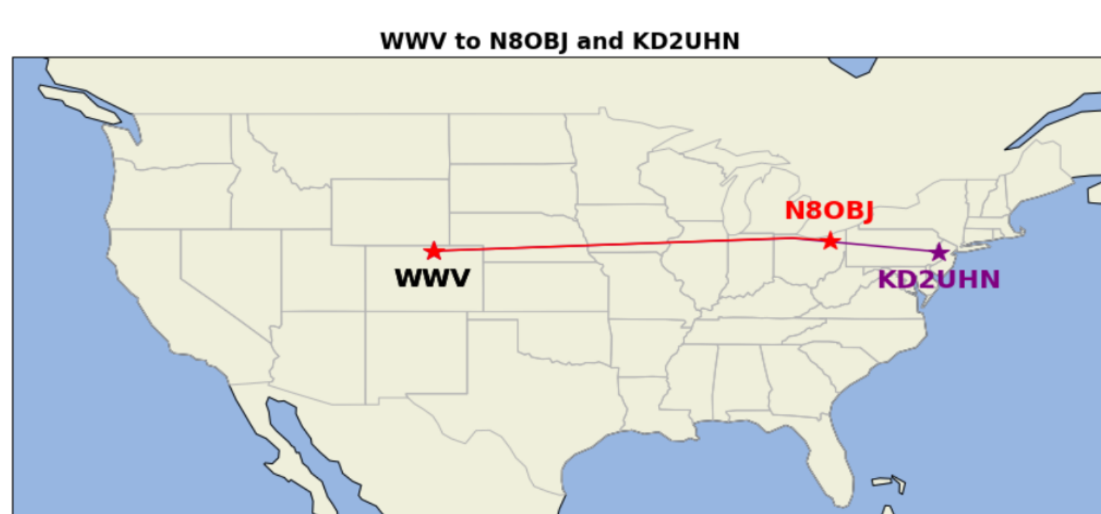
(FIGURE 1) The figure to the left depicts a map of a well-known United States Time Standard Station that transmits on extremely accurate frequencies (WWV) to 2 Grape Receivers discussed in this poster. There is currently a network of Grapes up and running across the USA, but the authors are particularly interested in these 2 due to their geographical locations, which are beneficial to studying the propagation direction of TIDs.
